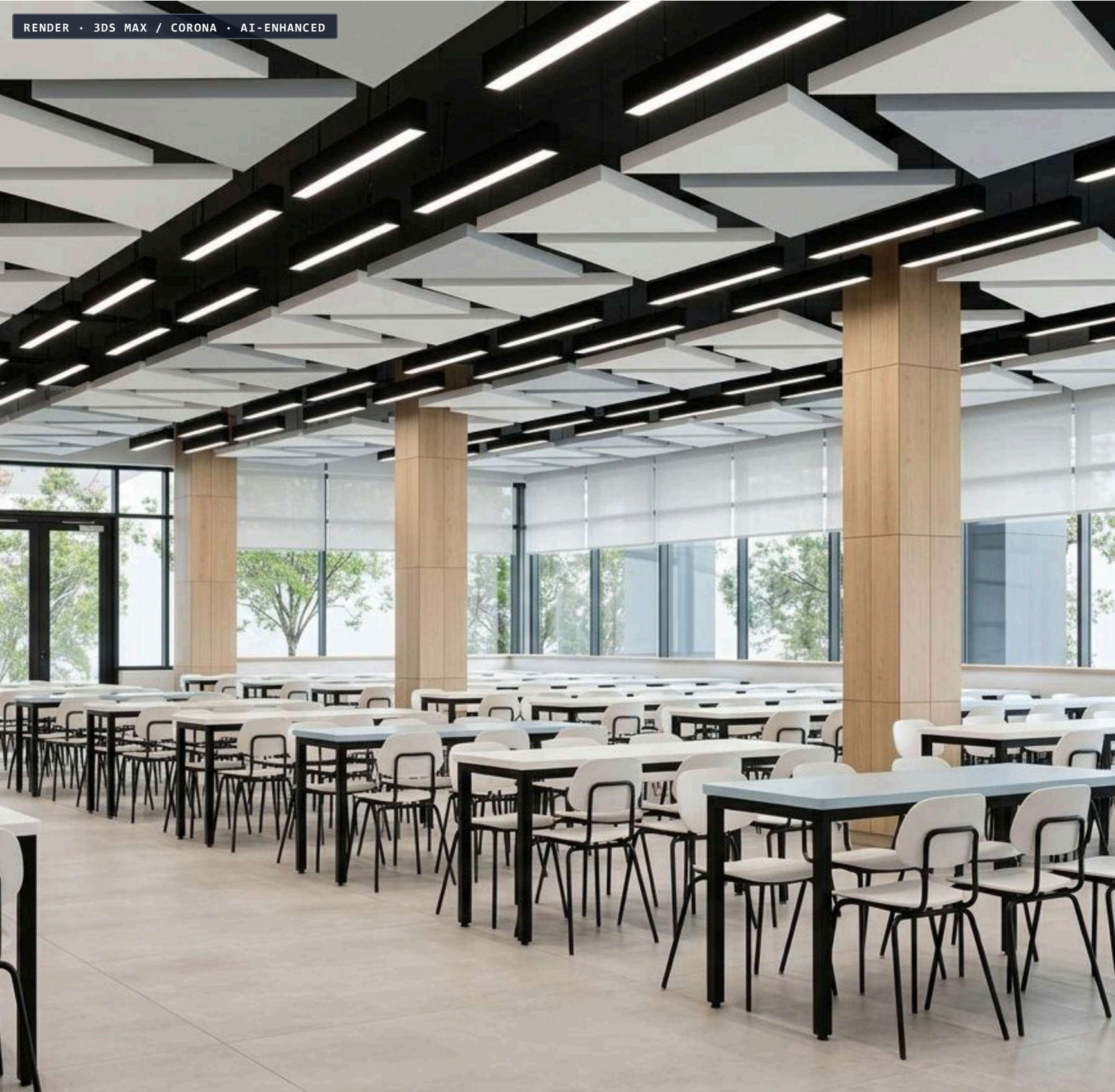
Fig. 09 — School Cafeteria: Geometric suspended drywall acoustic clouds, oak columns, and linear lighting.
